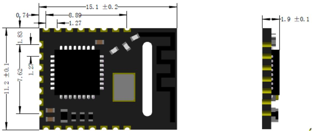
Fig4. Module Size Diagram
