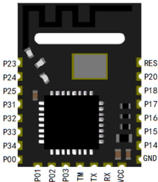
Fig. 2. Module Pins Distribution Diagram (Top View)
